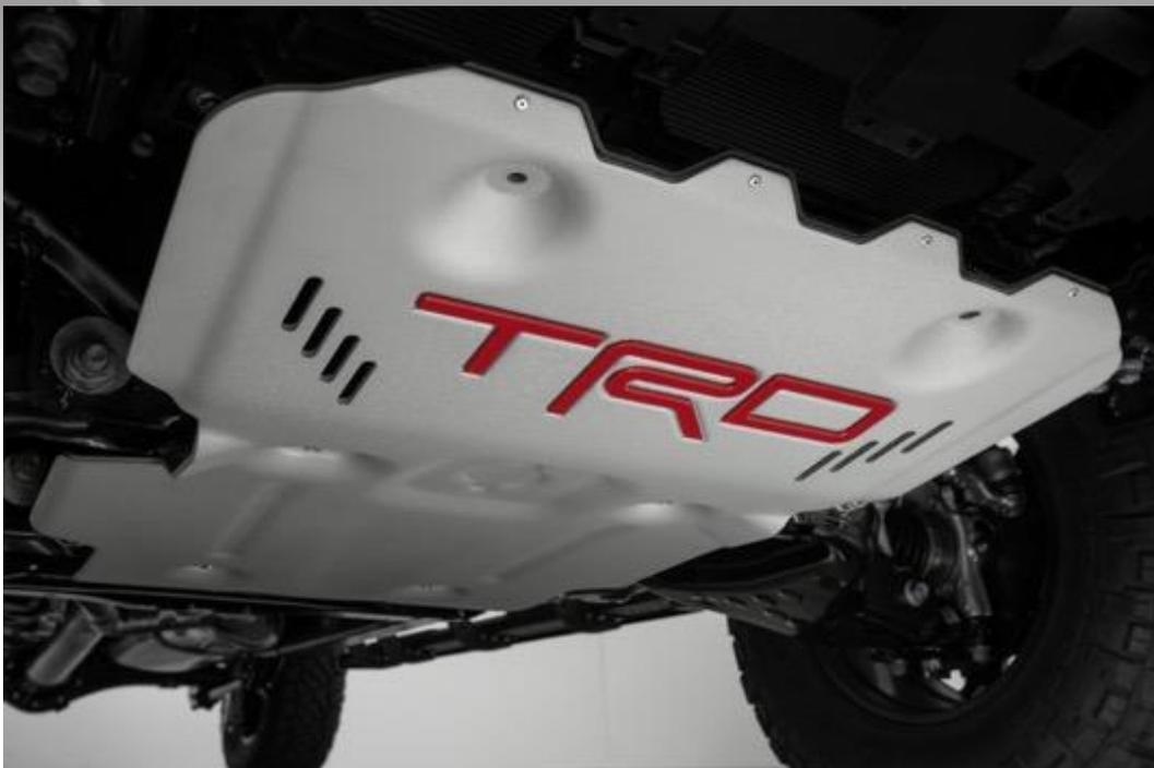
**Placa de deslizamiento TRD (Skid Plate)**
